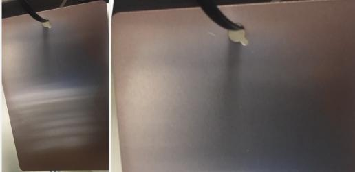
Day 10 (240 hours) – greater than 10% corrosion of both controls (panels A & B) - fail point
