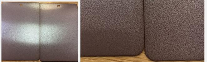
Day 93 (2230+ hours) – still less than 10% corrosion of the treated, panel C. Signs of corrosion seen around the edges of the Q-panel, and minor pock-marking in centre of plate. Corrosion covered less than 10% of the plate therefore fail point not reached but testing terminated.
