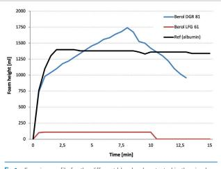
Fig. 1 Foaming profile for the different blends when tested in the circulation method (with circulation halted after 10 minutes). Albumin was used as foaming agent and the graph shows that Berol LFG 61 provides anti-foaming properties in this system, whilst Berol DGR 81 provides foaming
